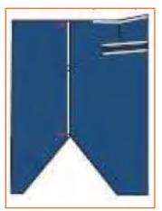
Turn the raw edges towards the left Step 4: side and put top-stitch at the edge of the back rise.
