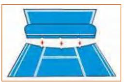
**Step 1:** Match the three notches on the neckband with the two shoulder seams of the body and the centre notch.
