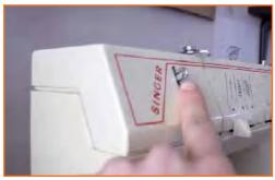
Then bring it down from the take up Step 5: lever into the coiled thread guide.
