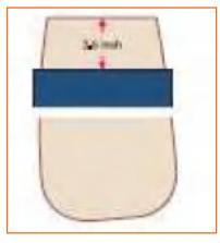
Step 18: Take the other piece of the pocket bag. Place the back pocket facing on top of the pocket bag at a distance of 2½ inches from top of the pocket bag.
