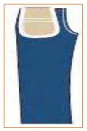
Put 1 cm stitch at the back rise starting Step 2: from top to bottom with back tack at both the top and bottom.
