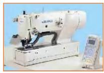
Fig:4.1.11: Button-hole machine
