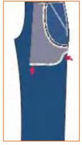
Step 7: Put 5 thread overlock stitches on the curved portion of the pocket bag.
