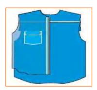
Step 2: The alignment should be such that the right side of the outer yoke piece faces the right side of the back piece of the shirt.
