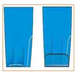
Make sleeve pleats by overlapping Step 2: the notches and stitching it in such a way that the pleats remain open from the edges.
