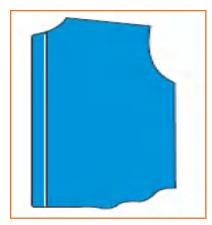
Start from the bottom and stitch the Step 6: inner side of the placket using edge stitch.
