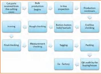
Fig.6.1.3: Sewing process flow
