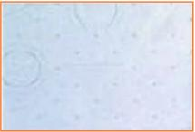
Fig.2.3.13(a): Ideal fusing in fabric
