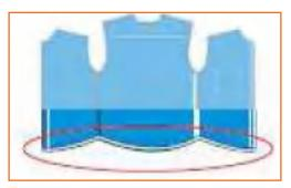
Step 2: • Fold the bottom (as per requirement) and put edge stitch from the left front side to the right side.
