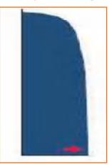
Take the fused J-fly piece and put Step 1: overlock stitch on the face side of the fabric starting from bottom of the curved side till the top.
