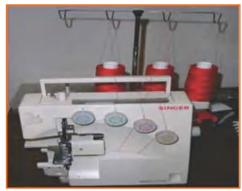
Fig:4.1.4: Over lock / over edge machine
