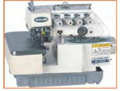
Fig:4.1.5: Three Thread Overlock Machine
