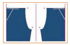
Take the fused J-fly piece and put Step 3: overlock stitch on the face side of the fabric starting from bottom of the curved side till the top.
