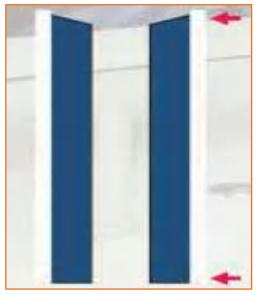
Step 1: Take both the upper facing pieces and put overlock stitch on the longer straight sides. Make sure the face side of the pieces is on top.
