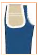
Now put overlock stitches at the back Step 3: rise starting from top to bottom.
