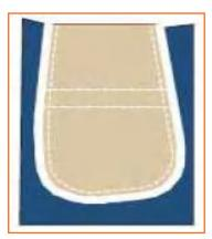
Step 22: Put 5-thread overlock stitches starting from right (back rise side) to the left side.
