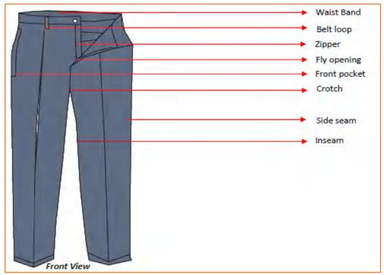
Fig.2.4.7: Front view of a formal trouser
