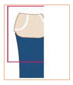
Step 2: Take the pocket bag and place it over the left front piece aligning with the mouth of the pocket.
