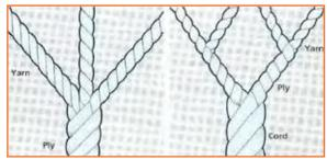
Fig.2.5.26: Ply and Cord of Thread
