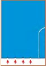
First, check that there are 4 notches Step 1: for sleeve pleatsand one notch at the centre of sleeve bottom.
