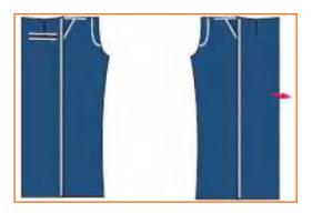
Step 3: Turn the raw edges towards the back. Put topstitches at the edge starting from top to bottom for the right side and bottom to top for the left side.
