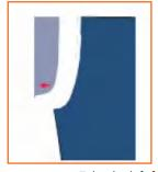
Take the left front piece and place the Step 4: J-fl y piece over the left front piece. Align the straight end of the J-fl y with the front rise along with the backside of the J-fl y facing up.
