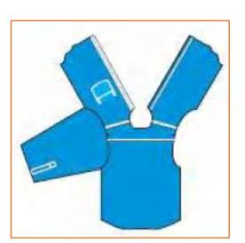
Step 6: Put an over-lock stitch at both the armholes. If top-stitch is required on the armhole, the sleeve should be kept up and the body part of the shirt should be kept down while putting the over-lock stitch. In case top-stitch is not required, the body part of the shirt should be kept up and the sleeve down.
