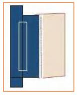
**Step 16:** Attach bone piece with the pocket bag using lockstitch.
