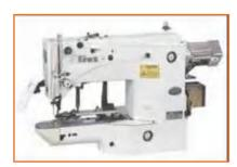
Fig:4.1.10: Button attach machine
