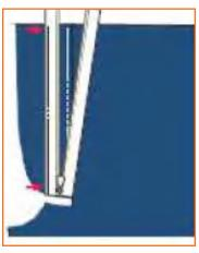
Place the zipper with slider facing Step 2: down over the fly piece at 8 mm from the straight edge at the top and 6 mm at the bottom. Align the bottom edge of the zipper with the curved portion of the fly piece.
