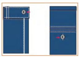
Step 1: Sew the button on the right hand side belt as per the design requirement and sew one button at the back pocket.
