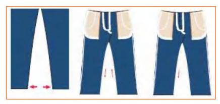
Put 5-thread overlock stitches starting from bottom to finish at other Step 5: bottom side.
