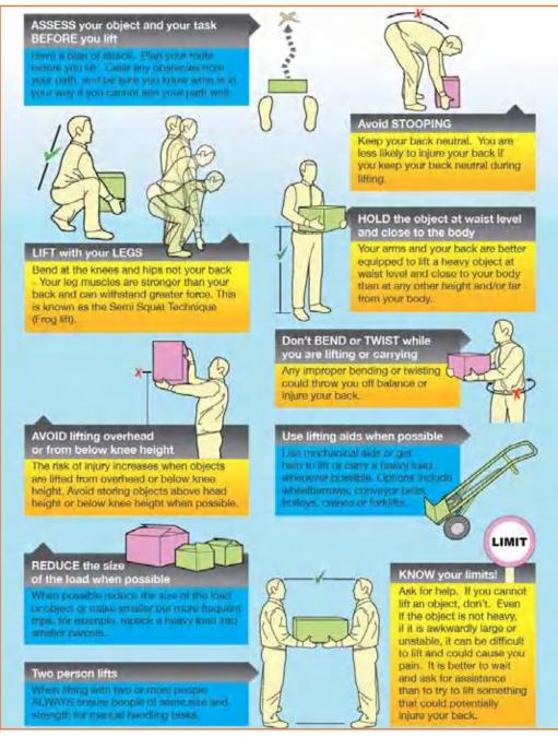
Fig.7.1.5: Do's and Don'ts in material handling
