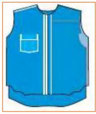
• The right side of the front and the right side of the back piece of the shirt are placed together by matching the yoke. The placket should be towards the centre.
