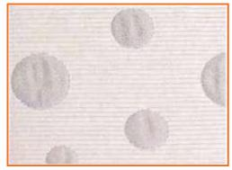
Fig.2.3.17(b): Fusing delamination
