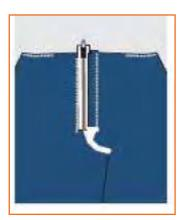
Step 11: Leave a gap of 1 mm between the zipper teeth and the edge of the fabric and put top-stitch.
