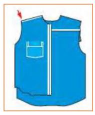
Step 3: The pieces are stitched at a distance of 1 cm from the edge leaving the bottom-most ply of the yoke.
