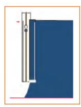
Turn the fabric and put edge stitch on **Step 7:** the zipper starting from bottom to top.
